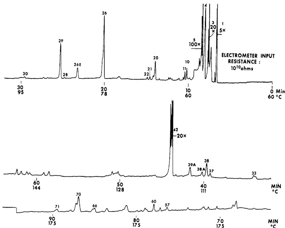
Figure 4. FID chromatogram of peel-oil-free orange juice vapor. Vapor sample size, 20 ml. Syringe injection. See other notes for Figure 3
