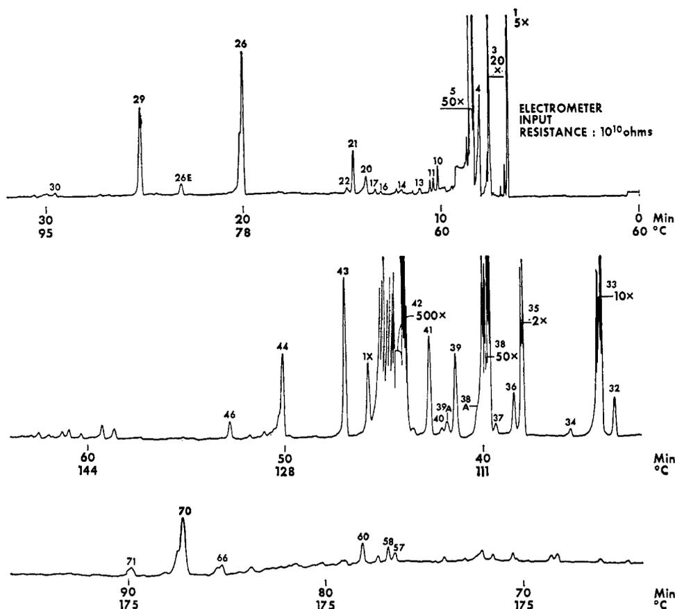
Figure 3. FID chromatogram of regular orange juice vapor. Vapor sample size, 20 ml. Syringe injection; water vapor not removed. Sensitivity 10 times that for Figure 2. Peaks are given the same number as the peak with the same relative retention in Figure 2
