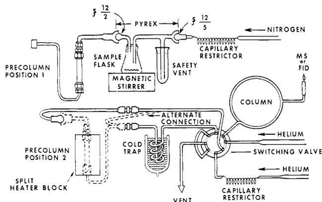
Figure 1. Apparatus for headspace analysis with water vapor removal
