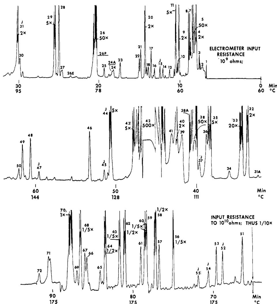
Figure 2. FID chromatogram of regular orange juice vapor. Vapor sample size, 1 l. Water vapor removed by precolumn system. Attenuation factors are as though this whole run was with electrometer input resistance at  $10^9$  ohms. Peaks are identified by number in Table II
